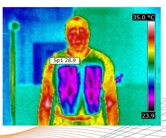
Environment temperature after 2 hours working in a CoolPax™ Cooling Vest
